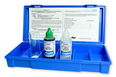
Taylor's K-1682 is useful for determining concentrations of six popular corrosion inhibitors, including morpholine.
