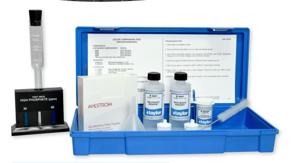
Tests utilizing the stannous chloride method for orthophosphate can be purchased as a stand-alone kit (K-1831 shown) or in combination with other boiler water tests.
