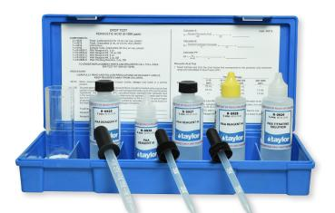
With the K-1546, the concentration of peracetic acid is determined by counting the number of drops of titrant needed to change the color of the sample water from deep blue to colorless and multiplying this by the factors provided in the instruction.
