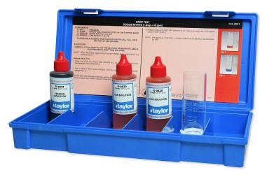
The drop-count titration in Taylor's K-1510 uses the "CAN" method (ceric oxidation of nitrite) to prevent interference in systems treated with glycol.
