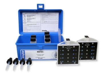
Unless the sample appears colored or turbid, a Midget comparator may be used to determine the concentration of metal in the water. K-1264 is shown.
