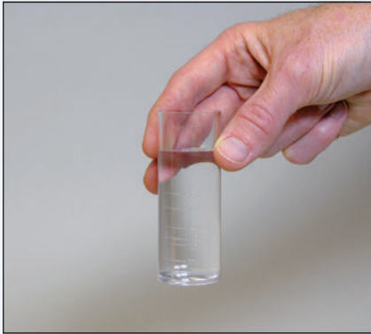
1. Rinse and fill #9198 sample tube with water to be tested in excess of desired volume.
