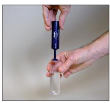
2. Orient SampleSizer for desired test volume: an arrow indicates the skinny end goes first for a 25 mL sample.
