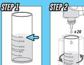
Rinse and fill sample tube (#9198) to 25 mL mark with sample water.
