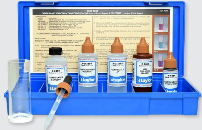
Use the K-1582 to ensure quaternary ammonium-based equipment/facility sanitizers do not exceed 200 ppm if you want to avoid a water rinse.
