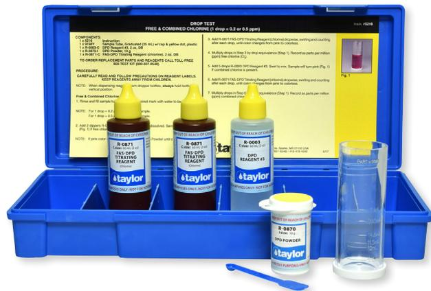
The drop-count titration in this FAS-DPD kit, K-1515-C, allows you to measure free and combined chlorine 0–20 ppm (in 0.2 or 0.5 ppm increments) without matching shades of pink. This is a boon for analysts with red-green colorblindness.
