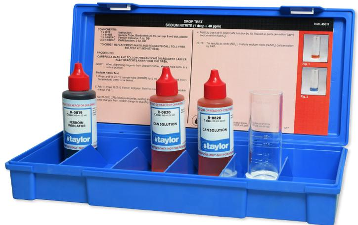
The drop-count titration in Taylor's K-1510 uses the "CAN" method (ceric oxidation of nitrite) to prevent interference in systems treated with glycol.
