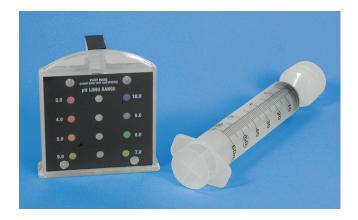
Midget comparators (#9052 shown) are the economical choice for monitoring pH when color and turbidity are absent. Use the syringe filter (#9803, right, plus appropriate size filter discs) to remove these interferences from your sample.
